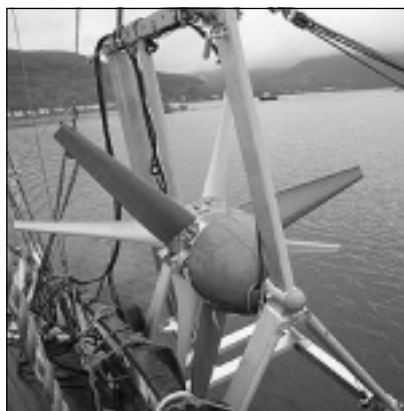
ESRU's contra-rotating marine turbine
