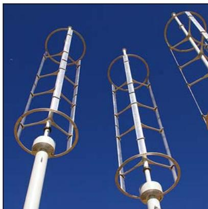
Vertical-axis wind turbines at a demonstration facility
