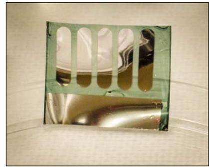
Solar cell fabricated on cellulose substrate
